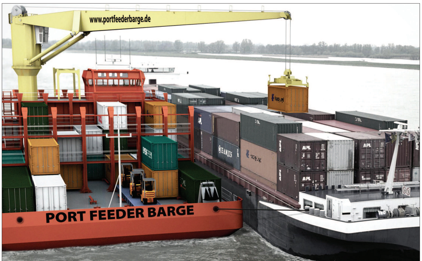
The Port Feeder Barge is serving an inland barge midstream (computer rendering)
