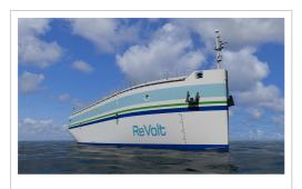
The unmanned battery-powered vessel ReVolt.
