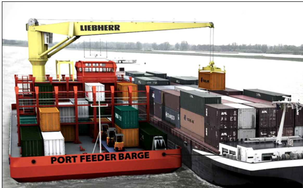
Fig. 7: The Port Feeder Barge is serving an inland barge midstream (computer rendering)
