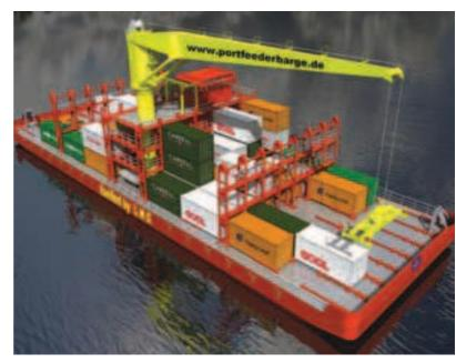
other half is not, enabling the vessel to also carry containers in excess of 40ft length as well as any over-dimensional boxes or even break-bulk cargo. 14 reefer plugs allow for the carriage of electrically driven temperature controlled containers.
