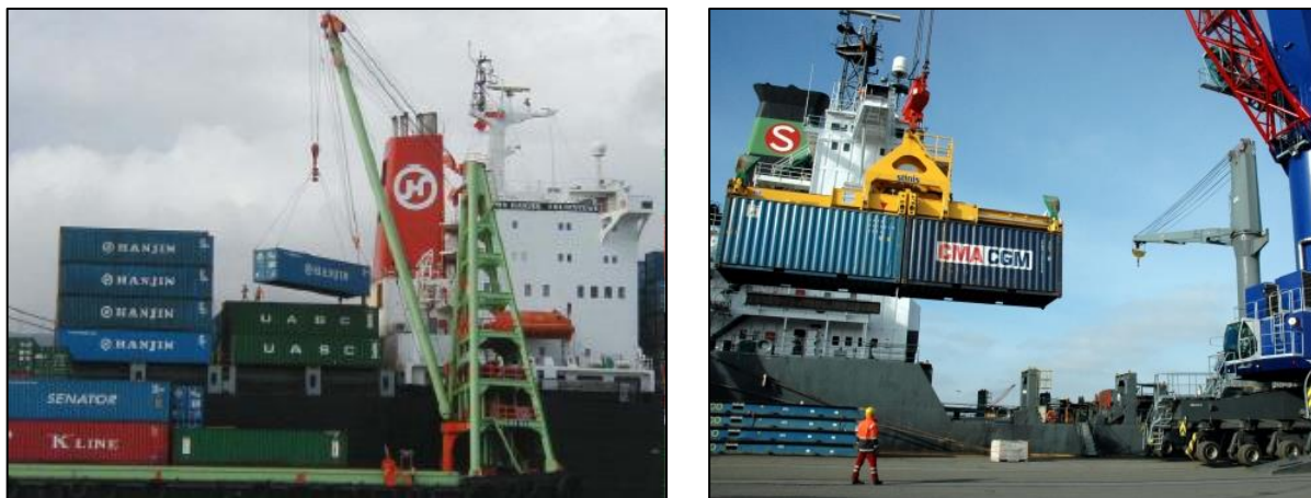
Figures 4 a & b: Midstream operation & twin lift tower spreader
