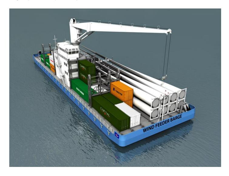
The Wind Feeder Barge can lift up to 100 tonnes using its onboard crane. Heavier cargoes can be loaded aboard via ro-ro operations.
