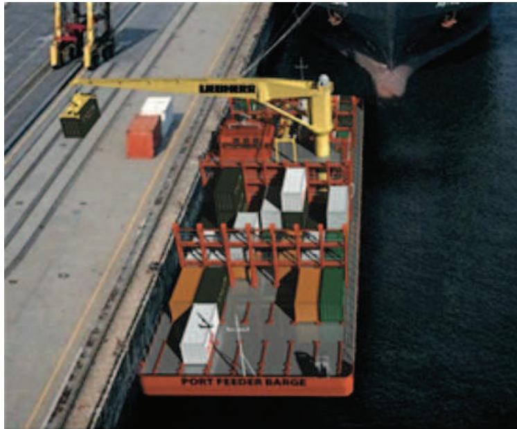
Fig. 20.3 The PFB is working independently from quayside equipment at a deep-sea terminal requiring only a small gap between two deep-sea vessels (artist impression)
