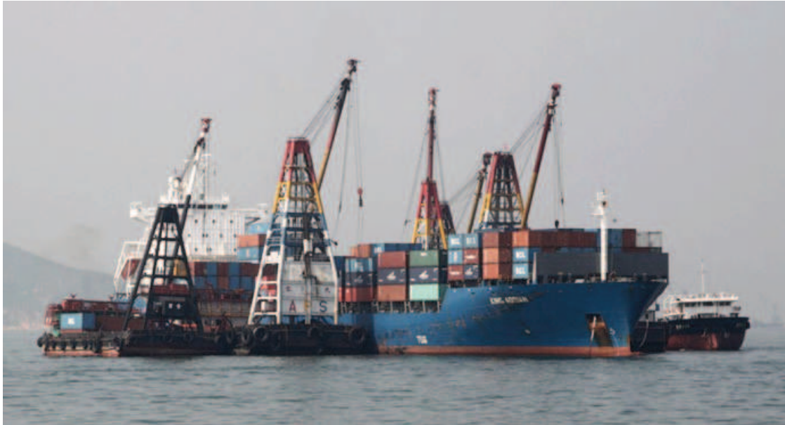
Fig. 20.8 Typical midstream operations in Hong Kong
